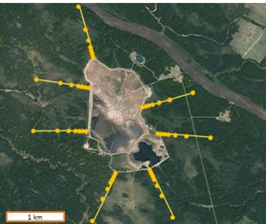
↑ Sampling around a mine site (Joutel), with data collection points, from 0 m to 1 km
